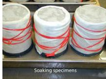
The capillary soaking process should be done by removing the specimens from the airtight bag, then removing the plastic wrapping. The specimens are wrapped with wet absorptive fabric and placed on a porous stone. The water level should reach the top of the stone and be in contact with the fabric wrap throughout the capillary soak process, but the soil specimen should not come directly into contact with the water.
