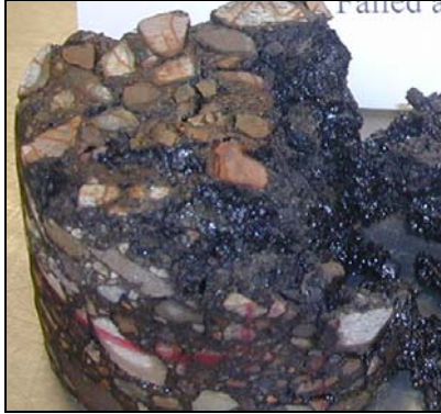
Liquid Mix - Core 6C (Failed after 19 Cycles)
